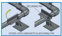
A bespoke locking system was supplied and attached to the concrete surround of the unit allowing the covers to be locked into place once opened by the site operative, therefore negating any issue of the covers falling and causing injury.
