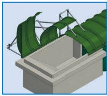
To avoid any health and safety issues such as the stairs becoming slippery, KEE designed and provided a bespoke extended cover arrangement over the pit access to the stairs. This extended cover set also incorporated the single operative lift metal framework system on the covers.
